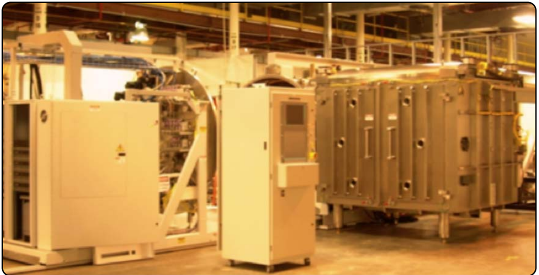
Figure 3 – Large-scale Sputtering Tool Capable of Processing 1 m Wide Web to be Installed at USPVMC Manufacturing Development Facility
